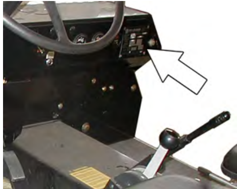
Data plate on the kick panel
