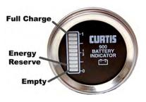
reset to fully charged only after a complete charge cycle is completed. A complete charge cycle is defined as battery voltage exceeding 2.35 volts per cell for a minimum of 6 minutes.
