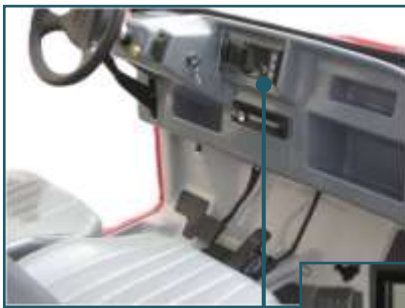
Radio, CD, MP3 Jack, Horn, Key Switch, Storage Space, Forward/Reverse Selector, and Hand Parking Brake
